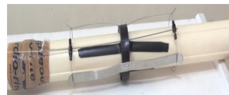
Magnet fixed with sealing tape; leaves compressed with release wire link and pulling cord
