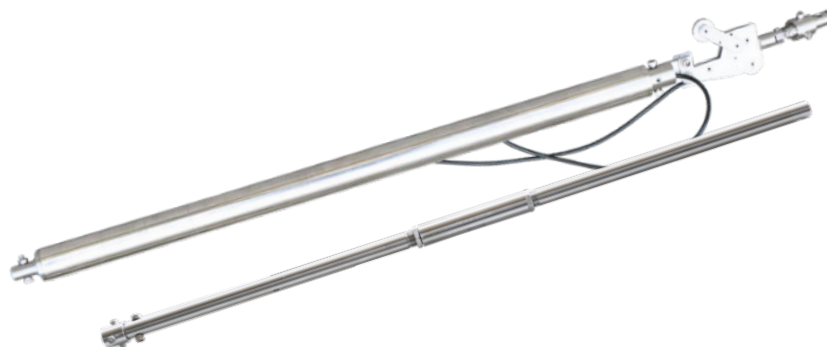
Figure 2-3 In-place 3D inclinometer system
