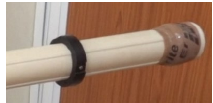
Figure 7-7 Datum magnet fixed on bottom most casing
