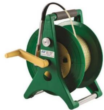
Figure 2-4 Magnetic settlement probe
